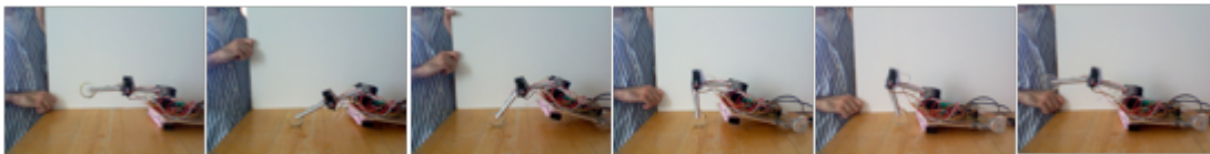
Figure 4.1: Time series pictures of the robot being controlled to crawl forward.
