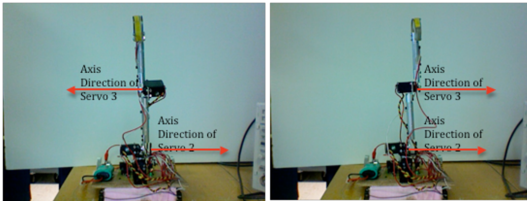
Figure 2.10: Comparison of the arm in a configuration where it is aligned and when it is not aligned.
