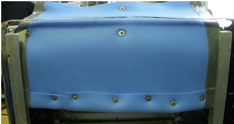
Figure 10. Riveted door on the oven.
