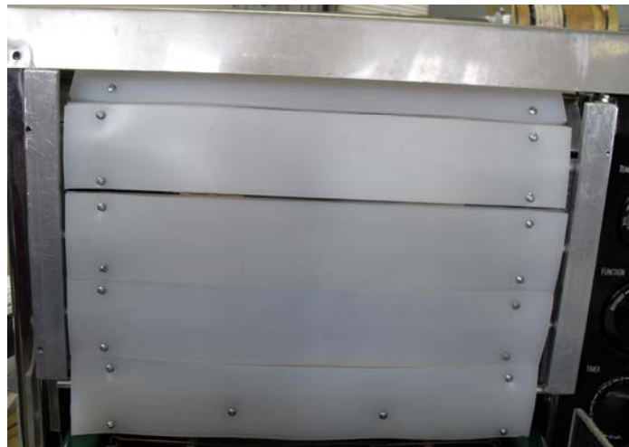
Figure 15. Prototype #4 showing gaps between hinged panels
