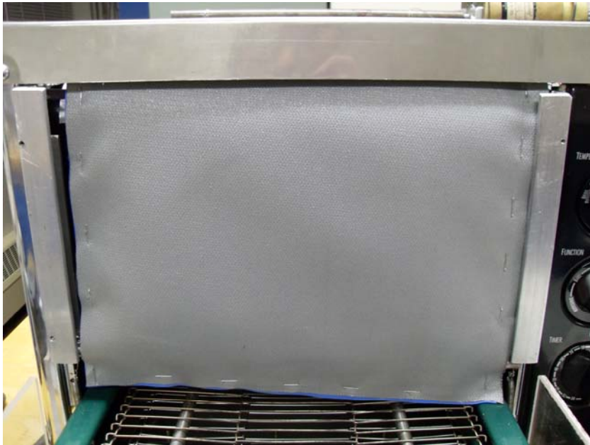
Figure 12. Final door used in oven with Pyroblanket™ on the outer layer
