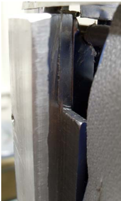
Figure 18. Guide channel with back edge cut off.
