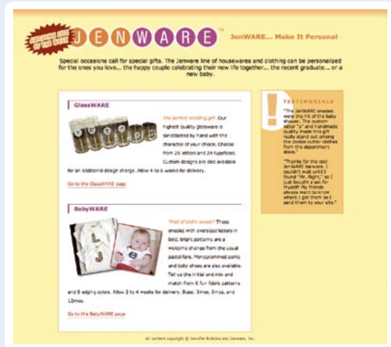
Figure 15-18. Two column format created by absolutely positioning the testimonials box.
