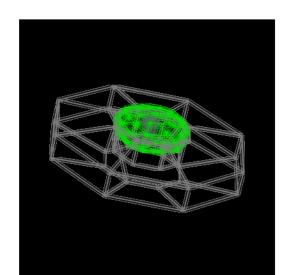
The bubble is actually a compressed sphere. We created triangularizations of cylinders and spheres at various levels of detail using a simple generating program, and then inserting them into our model file.
