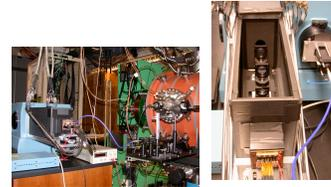
Figure 3: Left: Photograph of SSX lab showing vacuum chamber, monochromator, and associated IDS optics. Right: Overhead view of spectrometer exit slit, magnifying optics, and PMT array. The fiber optic carrying light to the entrance slit of the spectrometer is visible at right.
