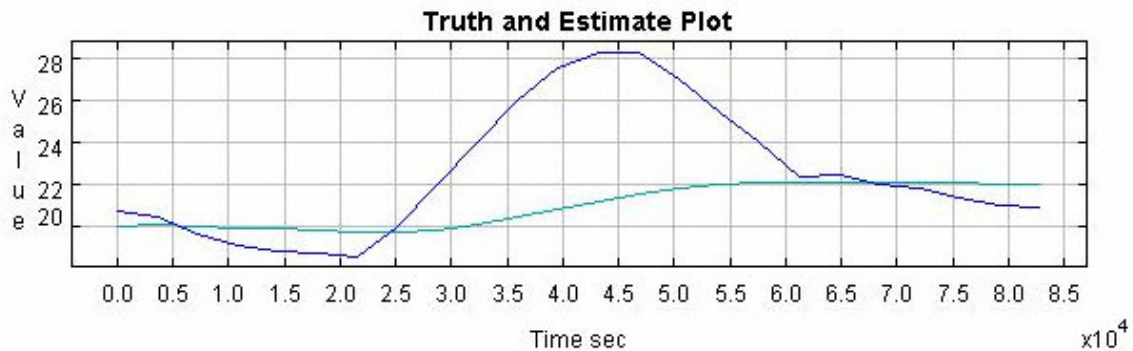
Figure 9: Temperature truth and estimate plot using Kalman filter in hour
