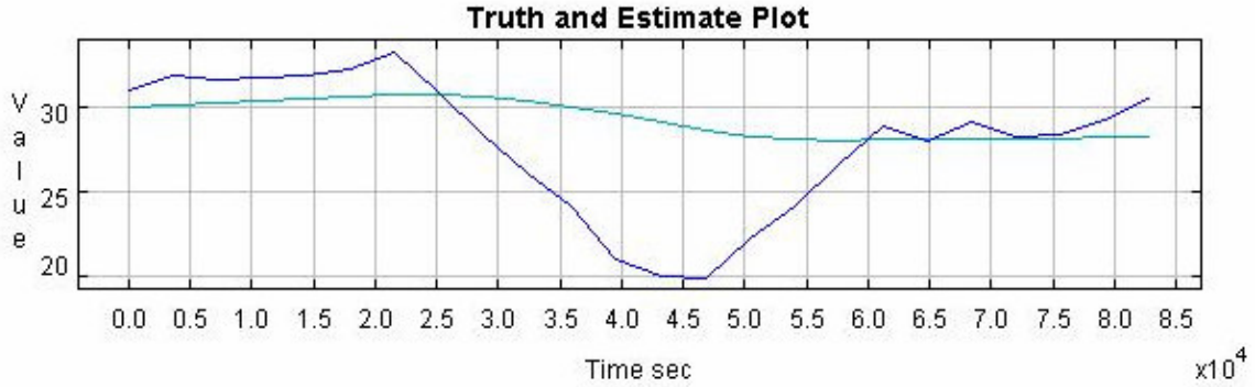
Figure 16: Humidity truth and estimate plot using Kalman filter in hours
