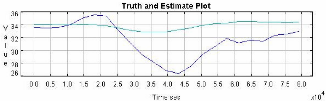
Figure 14: Humidity truth and estimate plot using regression with linear kernel
