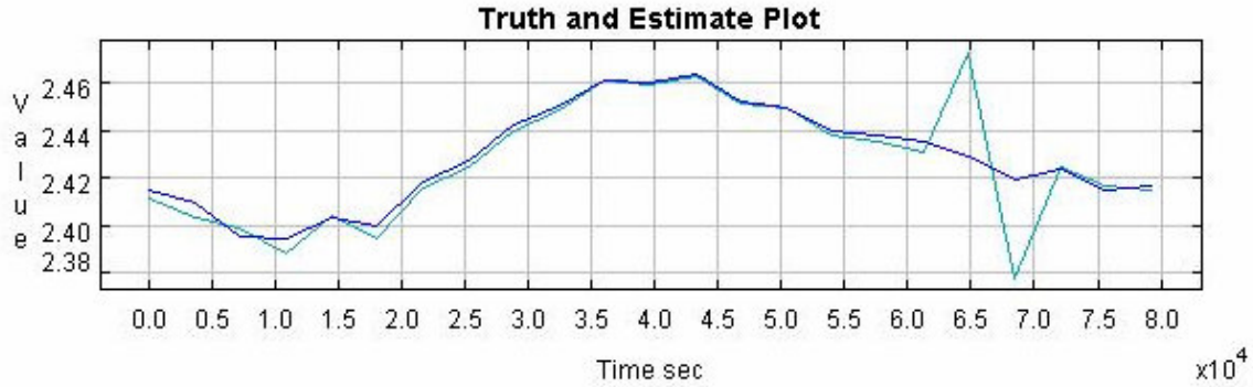
Figure 21: Voltage truth and estimate plot using regression with multi-quadric kernel
