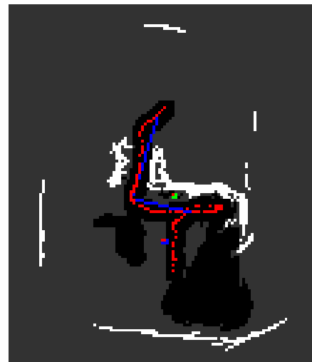
Figure 11: The robot, using AGG behavior, moves through a very tight gap to a goal beyond the obstruction
