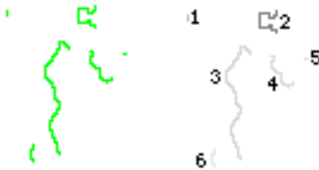
Figure 17: Left: The frontiers of the region. Right: The results of connected region extraction. The different connected regions are marked in different shades of grey, and numbered one to six.
