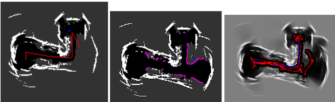
Figure 24: More results from the run begun in Figure 23. Left: When the hallway has been completely explored, a goal point is set that requires using Dijkstra's algorithm on the topological mapping to move back through known space. Middle: A goal point is set in the final frontier. Right: The final evidence grid
