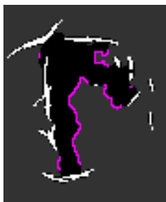
Figure 16: The shrunk image with frontiers found in pink (or light grey). The frontier processing had an occ_dist value of six
