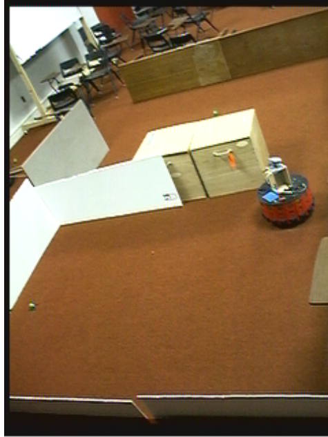
Figure 12: The robot using AGG moving through a gap to a goal point beyond the boxes. See Figure 13 for evidence grids from different behaviors in this scenario.
