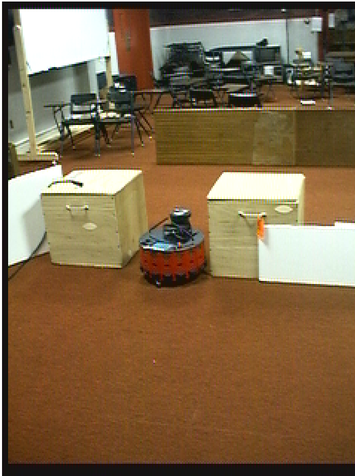
Figure 11: The robot, using AGG behavior, moves through a very tight gap to a goal beyond the obstruction
