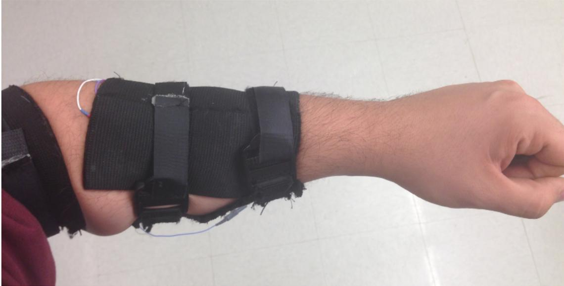
**Figure 3:** *Armband being worn for electromyography signal acquisition*
