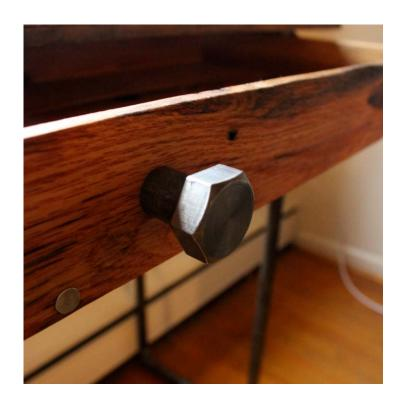
In 2011, I designed and built a side table for my girlfriend's apartment. The table was loosely based on the Maker Table developed by MAKE: magazine, but used hardwood from shipping pallets for the table surfaces and recovered cast-iron pipe fixtures for the frame, giving it a unique rustic-industrial look.
