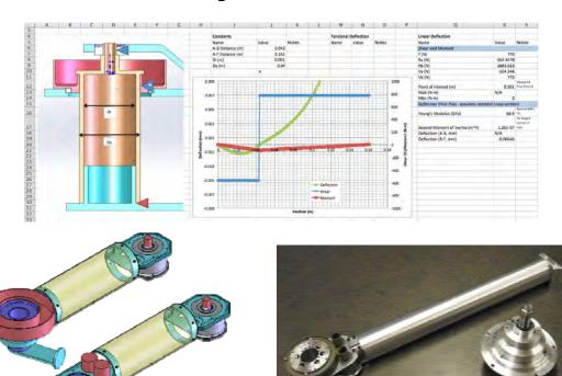
I was responsible for the high-level design of the Proficio's inner link and third joint. I considered a number of factors in my design study, including the aesthetics of the link, loads that the link's components would be required to withstand, and the design of the link's cable transmission. The images above show the progression of the link's design, from aesthetic concepts, to CAD mockups, to final product.
