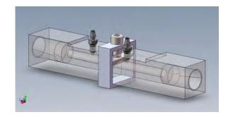
As part of my Fluid Mechanics course, I designed and built a wedge-type flowmeter to measure the flow rate of smoke through my Engineer's Hookah, below. After completing the on-paper design of the meter, I modeled and simulated fluid flow through the meter to check my calculations. I then fabricated the meter, developed an Arduino-based sensor apparatus to read the differential pressure produced by the meter, and built a housing for the electronics.
