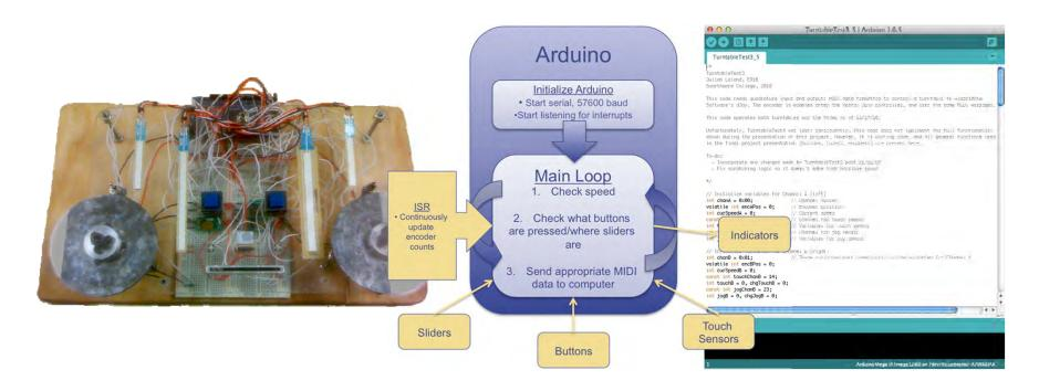
I developed a MIDI-based controller for the popular DJ application dJay as the final project for my Embedded Systems course. This project gave me an opportunity to become familiar interfacing with the many different sensors needed to simulate the wide range of input methods in the program, including touch potentiometers, capacitive sensors, powered sliders and high-resolution quadrature encoders.
