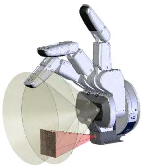
I am lead mechanical designer for the Barrett Perception Palm sensor suite for the BH8-series BarrettHand Manipulator. My responsibilities have included researching and sourcing components for the various sensor systems; developing a low-cost housing that retrofits to existing Barrett parts; developing a product BOM and manufacturing procedures; and directing a team of interns in integrating the system with the Barrett WAM arm.
