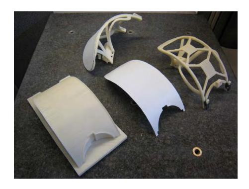
Because the Proficio is intended for in-clinic use, it must comply with robotic and medical device safety standards, including ingress and pinch protection. I was responsible for designing the cover systems that shield the internal drive components in the differential and the elbow, along with developing manufacturing processes and tooling for many of the prototype components.
