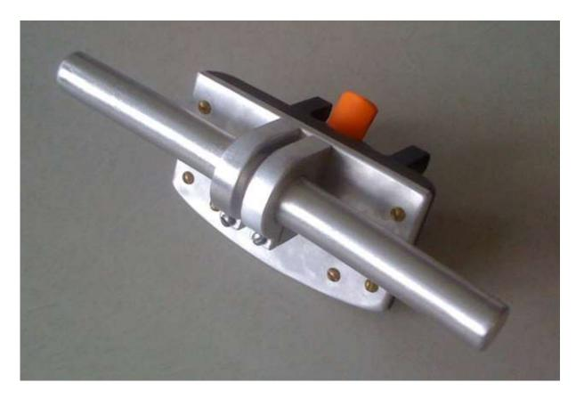
In the spring of 2011, a professor at Swarthmore College contracted with me to design and fabricate a light mounting bar for his bicycle. I designed the bar to be compatible with the existing Ortlieb mounting system the professor had installed; in addition to compatibility, I also had to consider the weight, corrosion resistance and aesthetics of the bar as factors in its design.
