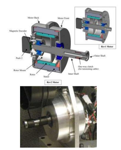
Motor Housing: I have designed multiple housings for the motors in the Proficio system, from early test prototypes through the final production design. I have also been responsible for extensive motor and transmission performance testing, and manufacturing process development.
