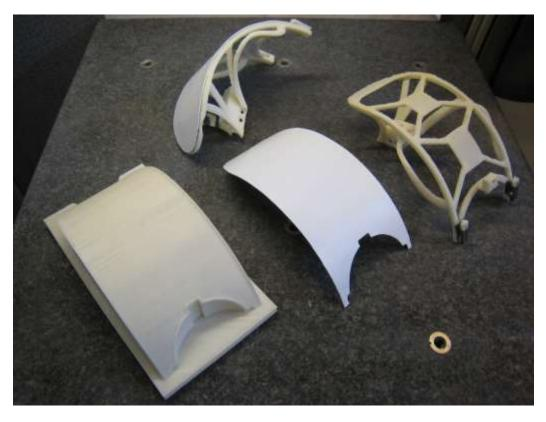
Cover Development: Because the Proficio is intended for in-clinic use, it must comply with robotic and medical device safety standards, including ingress and pinch protection. I was responsible for designing the cover systems that shield the internal drive components in the differential and the elbow, along with developing manufacturing processes and tooling for many of the prototype components.
