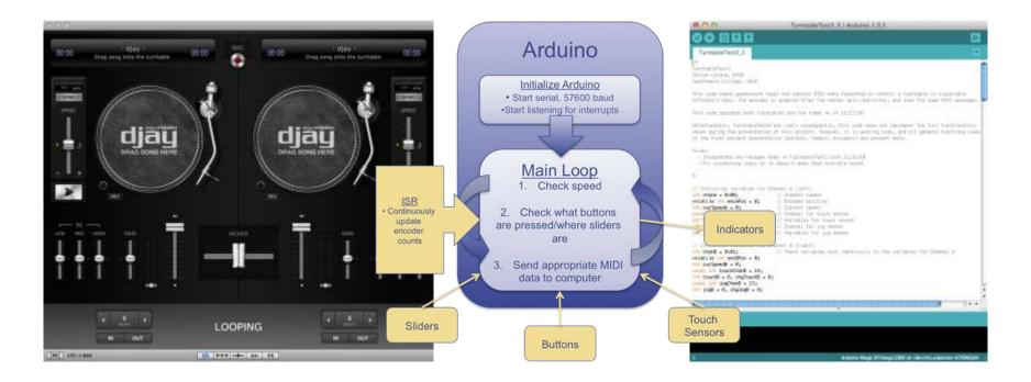
In the fall of 2010, I developed a MIDI-based controller for the popular DJ application dJay, as the final project for my Embedded Systems course. This project gave me an opportunity to become familiar interfacing with the wide range of sensors needed to simulate the wide range of input methods in the program, including touch potentiometers, capacitive sensors, powered sliders and high-resolution quadrature encoders.
