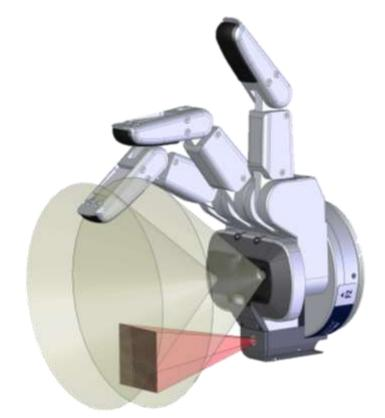
I was chief mechanical designer for the Barrett Perception Palm sensor suite for the BH8-series BarrettHand Manipulator. The Perception Palm suite incorporates dual cameras, infrared ranging and structured light projection and sensing directly into the palm of the manipulator.
