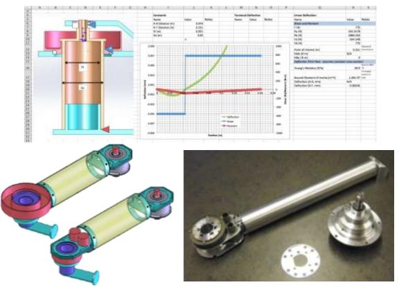
Link Design: I was responsible for the high-level design of the Proficio's inner link and third joint. I considered a number of factors in my design study, including the aesthetics of the link, loads that the link's components would be required to withstand, and the design of the link's cable transmission. The images above show the progression of the link's design, from aesthetic concepts, to CAD mockups, to final product.
