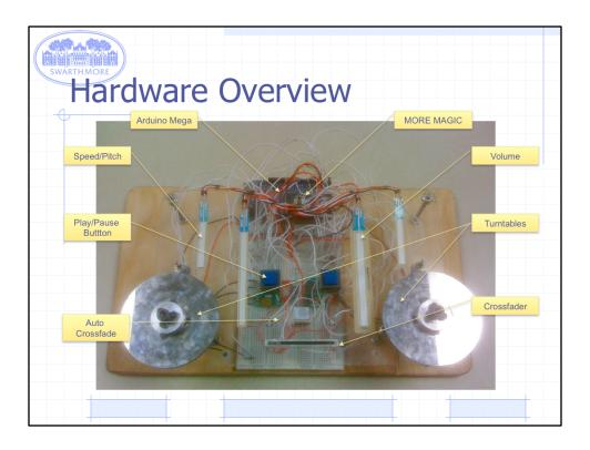
Turntables use capacitive touch sensors to detect touches on platters and on central hubs – platter scratches, hub seeks through song
