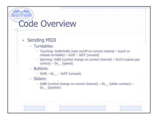
All data is sent via serial using Serial.print() command
