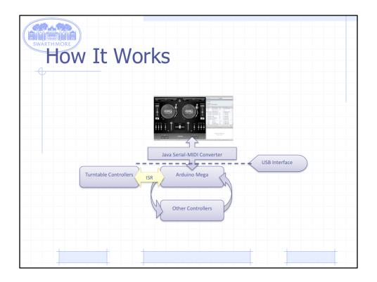
Serial to MIDI converter: takes data coming in to serial port through USB, and tells computer that it's MIDI data.
