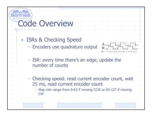
ISR method is higher resolution than simply looking at rising or falling edges.
