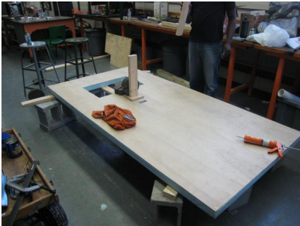
Figure 4: Deck after construction with lift and engine mount holes cut in it
