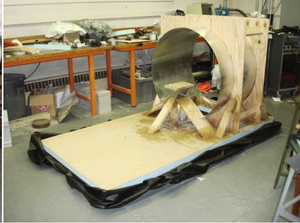
Figure 20: Completed skirt assembly
