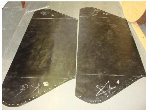
Figure 16: Front and rear skirt pieces after cutting
