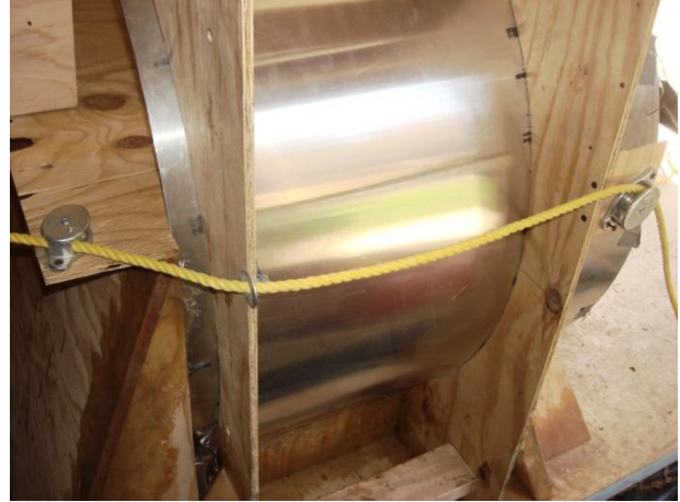
Figure 36: Side view of control system showing pulleys and rope
