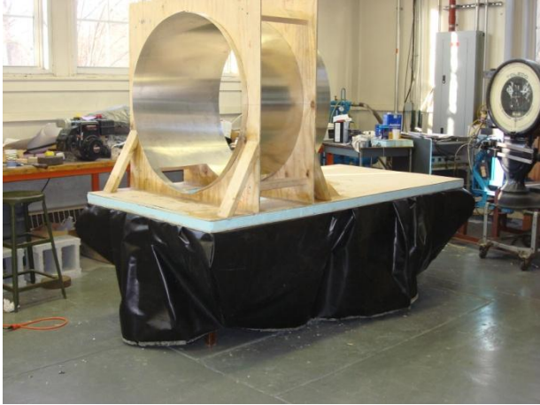
Figure 19: Skirt assembly after attaching outer perimeter to deck
