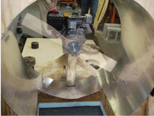
Figure 23: Testing of propeller in duct
