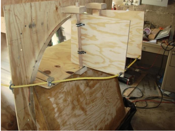
Figure 35: Rear view control system showing rudders, rope and pulley
