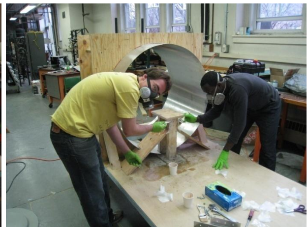
Figure 11: Fiberglassing engine mount supports
