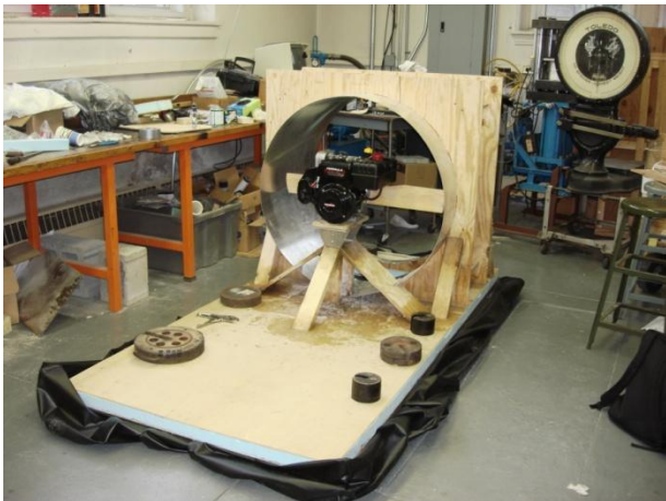
Figure 21: Engine and propeller mounted on engine stand
