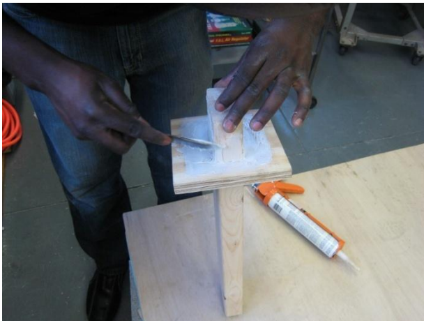
Figure 4: Applying adhesive to engine mount post
