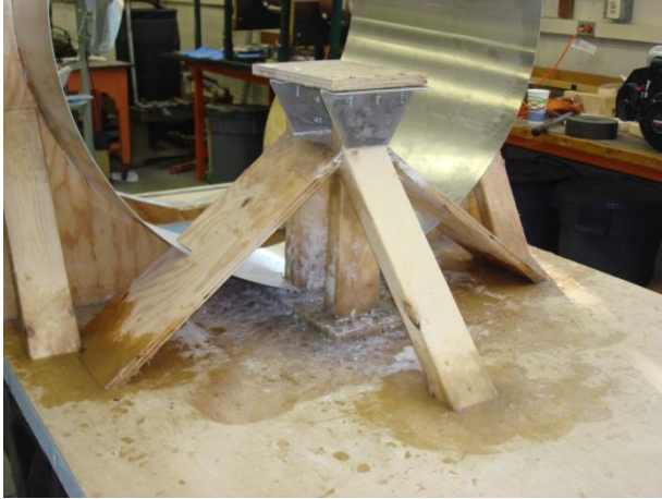
Figure 12: Engine mount supports after fiberglassing
