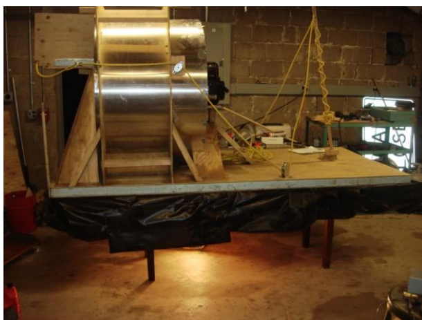
Figure 38: Skirt assembly after fixing unevenness in skirt profile
