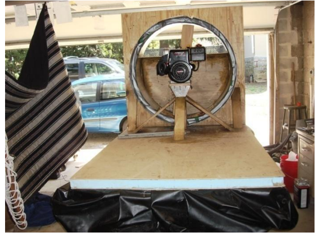
Figure 29: Front view of hovercraft after constructing air box
