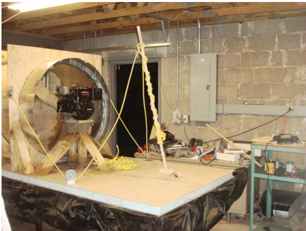
Figure 37: Front view of control system showing joystick, pulleys and rope
