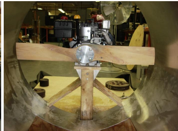
Figure 22: Testing propeller in duct
