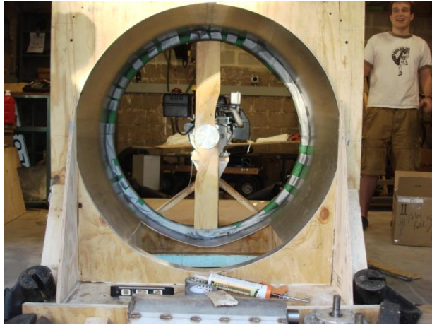
Figure 30: View of duct after clearance area was reduced.
