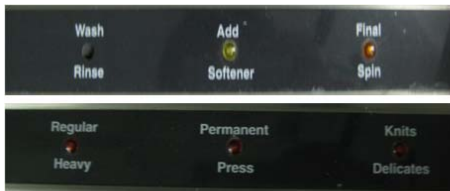
Figure 1. A picture of the LED indicator panels on washer and dryer. Top) Washer Display Panel, Bottom) Dryer Panel
