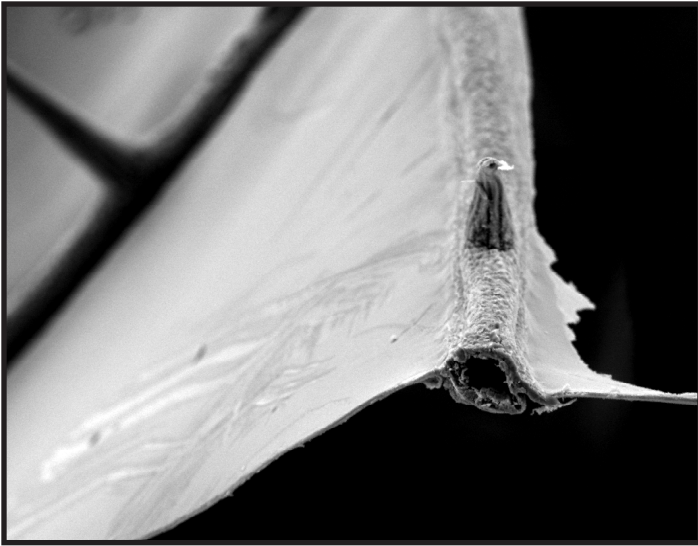
Figure 6. A scanning electron micrograph of the cross-section of a dragonfly longitudinal vein .
